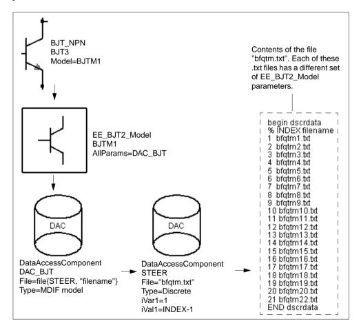
Note An assignment of the type:  $R1=file\{DAC1, "Rnom"\}$ , is equivalent to the expression  $R1=dep\_data(DAC1.\_DAC, "Rnom")$ .
