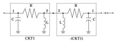
Another example is to de-embed the parasitics of the leads in a transistor. In the following illustration the base and collector parasitics are de-embedded to give just the chip BJT.
