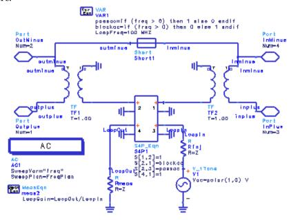
8. The large-signal loop gain mode is used to examine the behavior of the oscillator feedback loop as a function of frequency and injected voltage. It can be used to observe the compression of loop gain as the loop voltage is increased. In this mode, the OscPort2 element behaves as an analysis controller. Any simulation controllers should be disabled before using the OscPort2 in this mode. The
