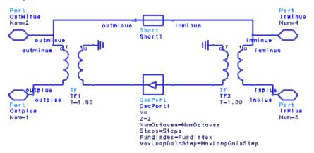
7. The small-signal loop gain mode is used to examine the small signal linear behavior of the oscillator feedback loop. In this mode, the OscPort2 element behaves as an analysis controller. Any simulation controllers should be disabled before using the OscPort2 in this mode. The analysis calculates and places in the dataset a complex value called LoopGain which is the small signal loopgain of the oscillator.
