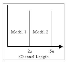
3. Depending on device size, one of the multiple models should be selected for a device at simulation time. If device size needs to be varied over a certain range, manual model change for each new device size would be very cumbersome. The
