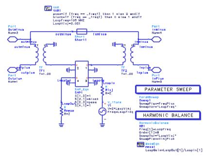
In both small signal and large signal loop gain modes, this element injects a test signal into an oscillator circuit for stimulating oscillations. The specialized directional coupler has zero electrical length and is invisible to normal circuit simulation. It injects a fundamental frequency test signal, blocks the fundamental frequency flow in the feedback path, monitors the signal returned by the feedback path and calculates the loop gain.
